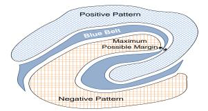
Figure 1. [Best Viewed in Color] Demonstration of Nonlinear Maximuum Margin Classification: Any separating boundary within the blue belt achives the maximum margin.
